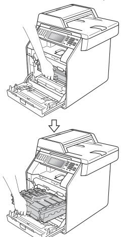
9 Turn the green lock lever (1) at the left of the machine counterclockwise to the release position. Holding the green handles of the drum unit, lift the front of the drum unit and remove it from the machine.
